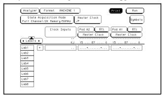
**c** Press the Trigger key. Make sure pattern term **a** is "A". If not, select the field next to "a" under the label Lab1. Type "A", then press the Select key.
